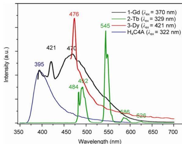
**Figure 9** Luminescent spectra of **1–3** and H<sub>4</sub>TC<sub>4</sub>A in the solid state at room temperature.
