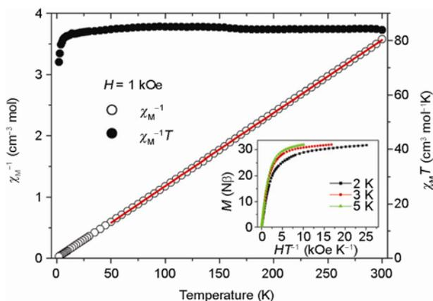
**Figure 5** Plots of  $\chi_M T$  vs.  $T$  and  $1/\chi_M$  vs.  $T$  for **3** in a 1 kOe field. Red line represents the Curie-Weiss fitting. Insert:  $M-HT^{-1}$  plot of **3** at 2, 3 and 5 K.
