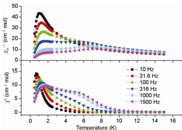
**Figure 7** Temperature dependence of the in-phase (top) and out-of-phase (bottom) components of the ac magnetic susceptibility for **3** in a zero dc field.
