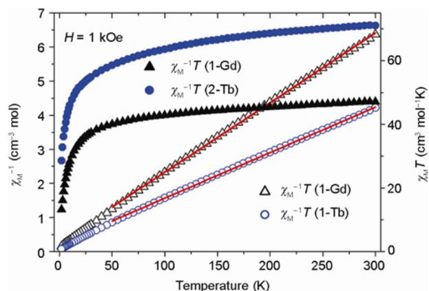
**Figure 4** Plots of  $\chi_M T$  vs.  $T$  and  $1/\chi_M$  vs.  $T$  for **1** and **2** in a 1 kOe field. Red lines represent the Curie-Weiss fitting.
