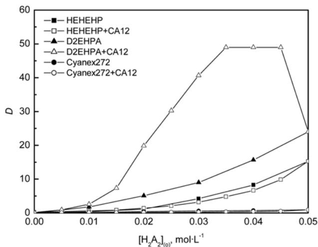
**Fig. 4. Extraction of  $Y^{3+}$  with organophosphorus acids and their mixtures with CA12:  $[Y^{3+}] = 5.0 \times 10^{-3} \text{ mol} \cdot \text{L}^{-1}$ ,  $\text{pH} = 3.0$ ,  $\mu = 0.6 \text{ mol} \cdot \text{L}^{-1}$ ,  $[H_2A_2] + [CA12] = 0.05 \text{ mol} \cdot \text{L}^{-1}$ .**
